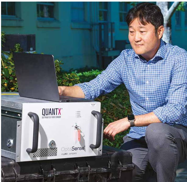
Gene Ichinose, a seismologist at Lawrence Livermore National Laboratory, looks over an interrogator, an instrument that allows buried fibre-optic cable to be turned into thousands of virtual seismometers
