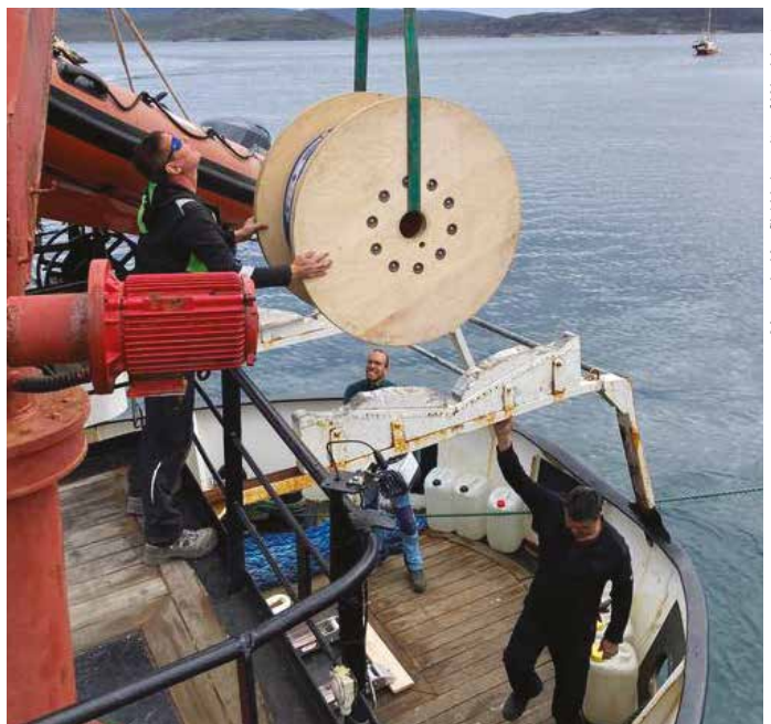
University of Washington’s Dominik Gräff and two crew members load the fibre-optic cable onto the back of the research vessel Adolf Jensen
