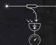
Optical Power Tap Monitor
