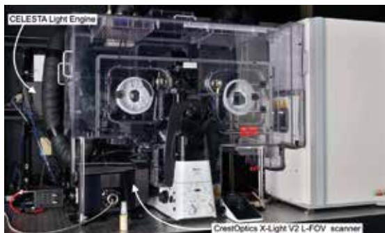
(Figure 3:) Instrumentation for automated three-dimensional imaging of living cells. The system is a Nikon Ti2 inverted microscope equipped with an environmental enclosure for maintenance of cellular homeostasis. On the right is an incubator for storage of live cell arrays, before and after analysis. To the rear, left of the microscope is the Lumencor CELESTA light engine
