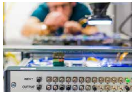
QuiX Quantum's photonic processor enables users to perform arbitrary, controlled interference between a number of optical channels, in the classical or quantum domain
