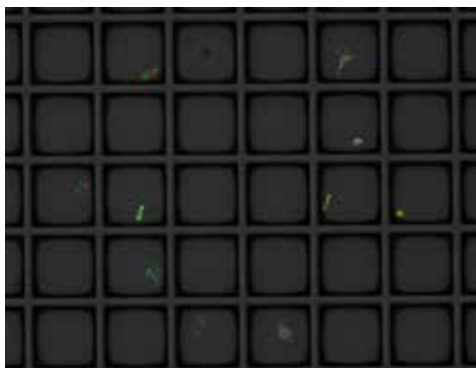
(Figure 2:) Cellular phenotypes displayed on a 6x5 micrafft array. Each 100µm square raft consists of magnetic polystyrene embedded in a polydimethylsiloxane (PDMS) substrate
