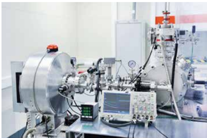
At Fraunhofer ILT, a laboratory system for EUV has been built to process wafers with a diameter of up to 100mm
