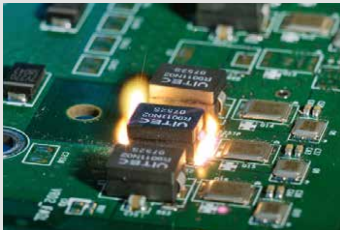
Lasers can recover valuable raw materials from end-of-life devices
