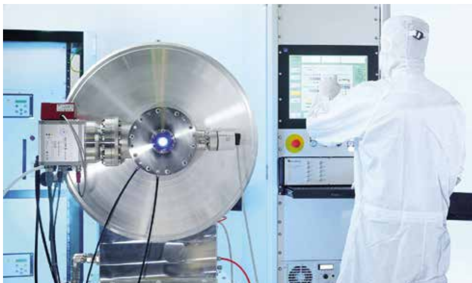
The EUV source at Fraunhofer ILT's Excimer facility delivers 40W at 13.5nm
