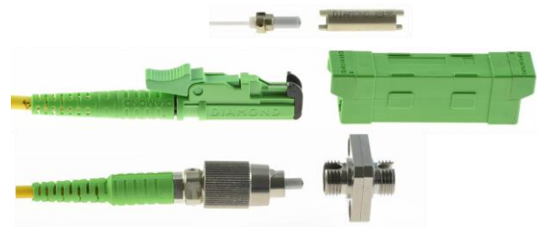
Figure 4. Examples of DMI (top), E-2000™ (middle) and FC (bottom) connectors with the corresponding mating adapters. DMI and FC connectors rely upon alignment keys based upon a notch-slots combinations, while the E-2000™ relies upon its rectangular cross section.
