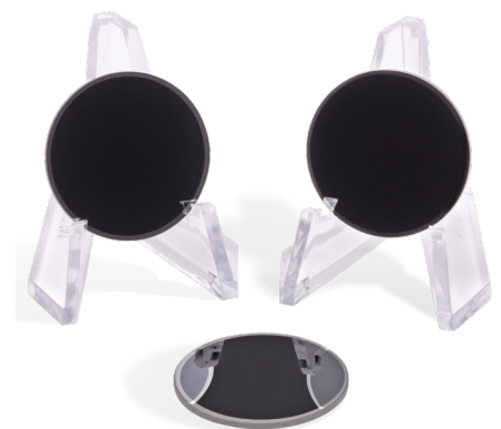
Witness samples of DLC-coated optics
