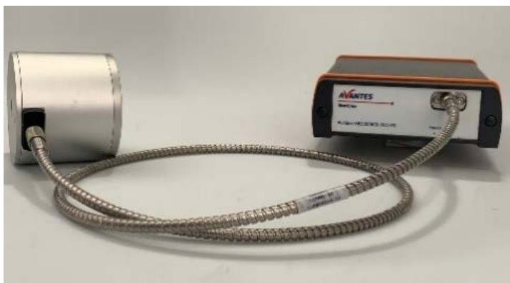
Figure 4. Setup with AvaSpec spectrometer, fiber-optic cable and integrating sphere
