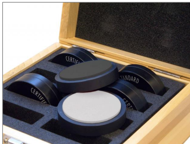
Figure 8: Spectralon Calibrated Diffuse Reflectance Standards
