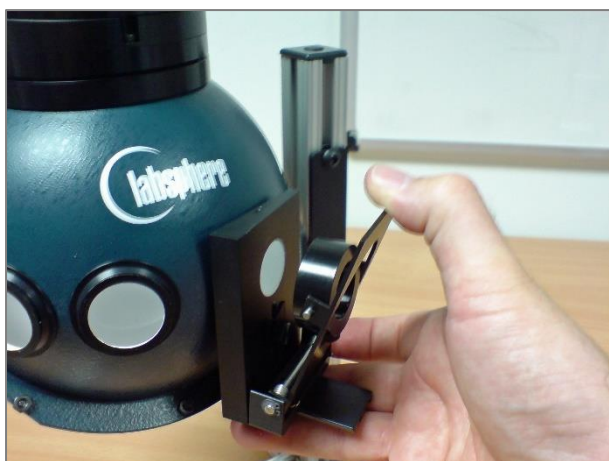
Figure 7: Labsphere Reflectance Measurement Integrating Sphere
