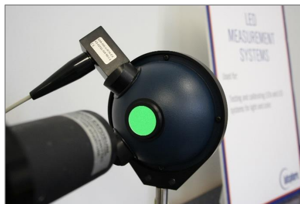
Figure 5: Labsphere Integrating Sphere Radiometer
